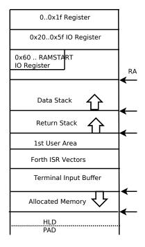
Fig. 3.4: Alternative RAM Structure
